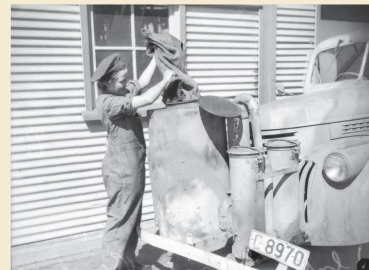
The hopper of a gas producer attached to the front of a utility being filled with charcoal. The utility was at Flinders Naval Base, Victoria. Photo Australian War Memorial.
